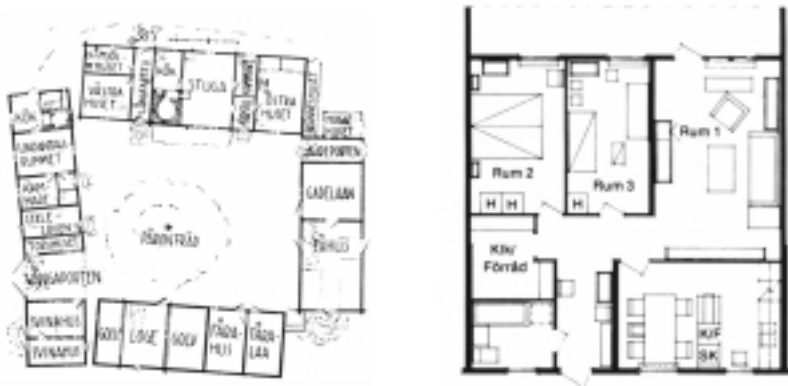
Fig.1. Plan of a Swedish farm with spaces for the majority of the household's activities spread out in different buildings united in one physical form.
