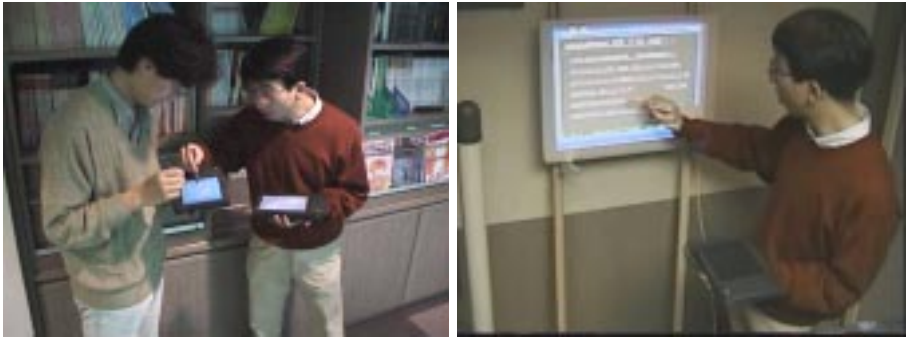
Fig. 4. Applications of Pick-and-Drop (left: transferring data between two PDAs, right: picking up information from the kiosk terminal)
